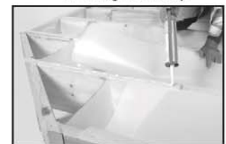
Caulk wherever downspout or troughs overlap
